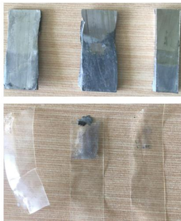
Fig 5. Cross-Hatch Tape Test Results According to ASTM D3359.
