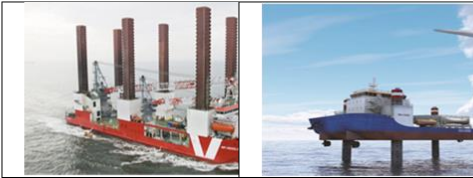
Fig. 2. Offshore Wind Turbine Installation Jack-up Vessel
