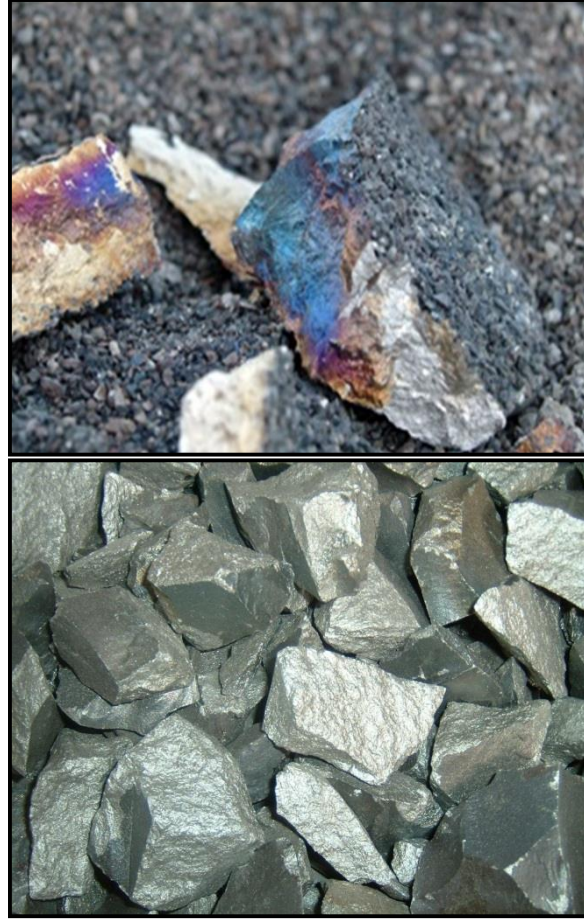
Fig. 2. a, b- Ferrochrome alloy (FeCr), Ferrochrome pieces in bulk
